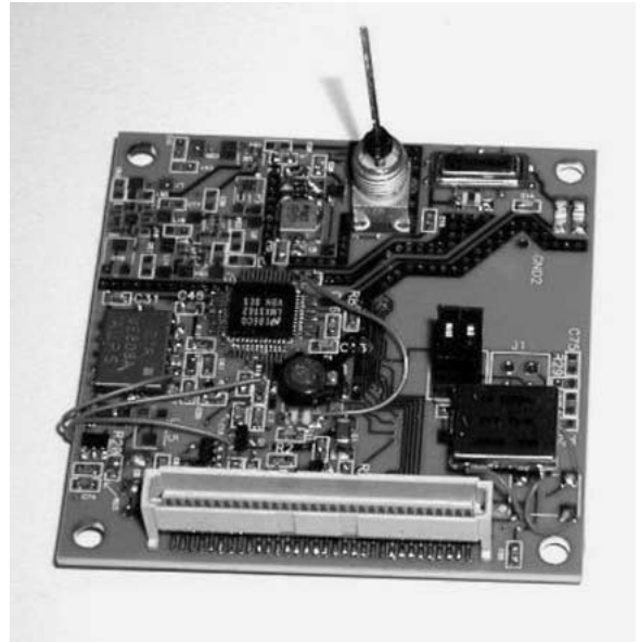
Figure 6. The \mu\text{AMPS} Radio. This radio is designed to stack onto the main \mu\text{AMPS} processor board (not shown).
