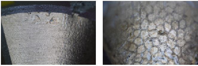
Figure 1. Corrosion of the copper plate due to distilled water seeping through the protective layer in the prior art sensor. Initial (left); after 2 weeks (right).
