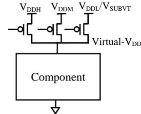
Figure 1. Architecture for using headers to implement DVS across a wide voltage range.
