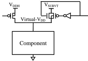
Figure 8. Proposed transmission gate power switch
