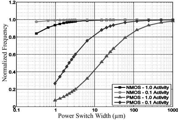
**Figure 4. Simulated Frequency at 0.3V for the conventional PMOS and proposed NMOS**
