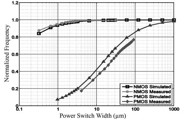
**Figure 7. Simulated and Measured Frequency at 0.3V with an activity factor of 1.0**
