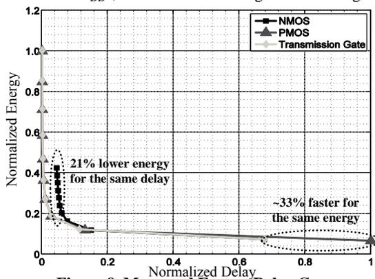
Figure 9. Measured Energy Delay Curves
