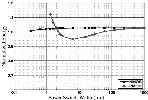
**Figure 5. Normalized Energy per op vs. power switch width**
