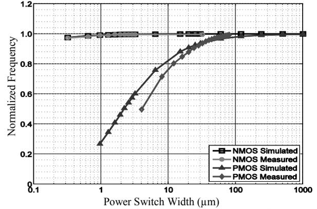
**Figure 6. Simulated and Measured Frequency at 0.3V with an activity factor of 0.1**
