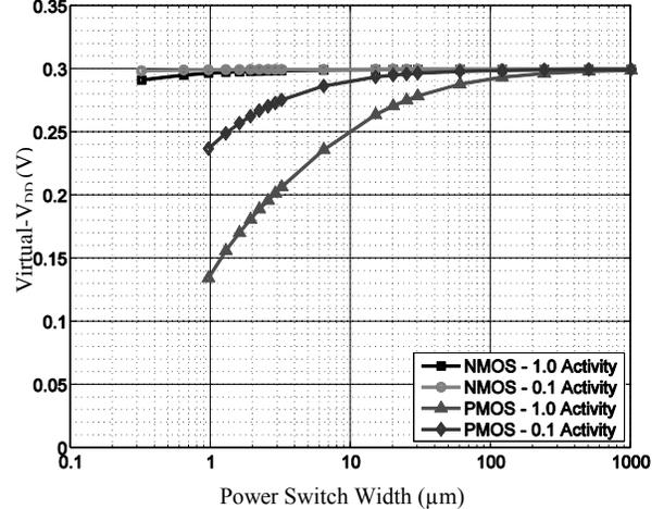
**Figure 3. Simulation Virtual- $V_{DD}$  at 0.3V for the conventional PMOS and proposed NMOS**
