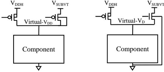
**Figure 2. (left) Conventional PMOS subthreshold power switch (right) Proposed NMOS subthreshold power switch**
