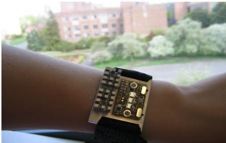
**Figure 3: Our prototype body-worn solar/thermo-electric generator for health monitoring applications.**
