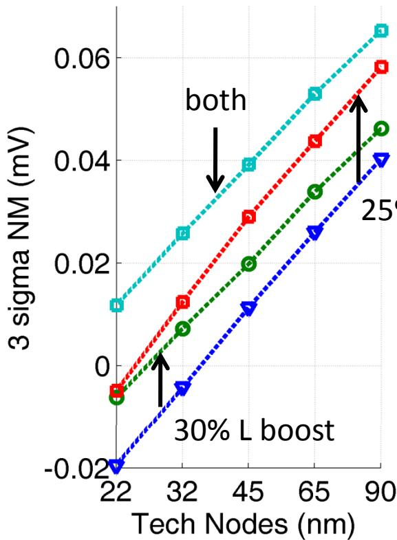
$V_{DD}$  boost and L increase help NM and reduce variability
