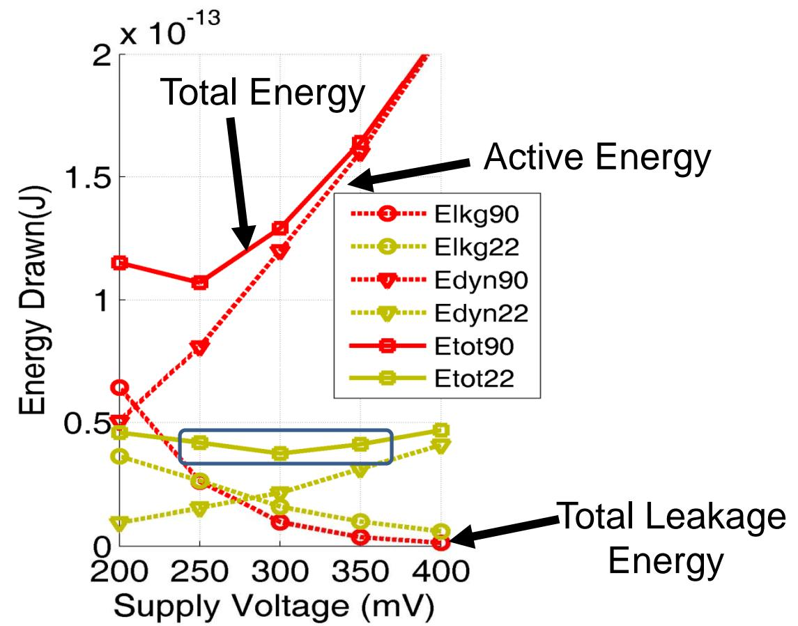
Scaling reduces  $E_{\min}$ , and raises  $V_{\text{opt}}$
