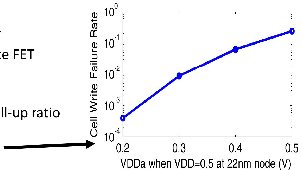
Bitcell  $V_{DD}$  collapse gives adequate writability to 22nm
