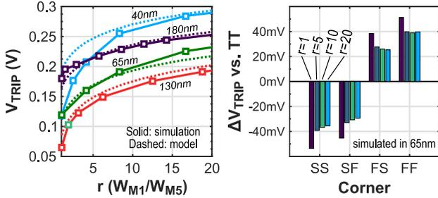
Fig. 3. Modeled and simulated DLS inverter logic threshold  $V_{TRIP}$  versus sizing ratio of  $M_1$  and  $M_5$  for multiple technologies in the TT corner (assuming a device selection such that  $V_{th0,M1} < V_{th0,M5}$ ), and impact of process corner on  $V_{TRIP}$  value for different sizing ratios.
