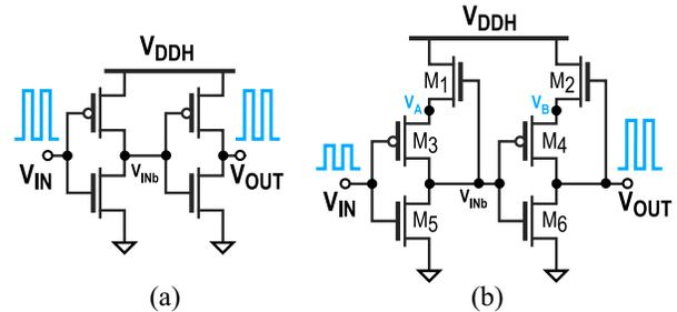
Fig. 1. Schematic of (a) traditional digital buffer and (b) proposed level converter.
