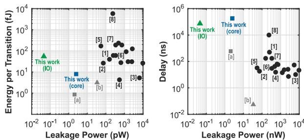
Fig. 10. Comparison with the existing level converter designs (shown by dark markers). As an added reference point for comparison, markers [a] and [b] show the performance of traditional digital buffer standard cells [from Fig. 1(a)] in the same 65-nm technology under normal operation at 0.3 V and 1.2 V supplies, respectively.
