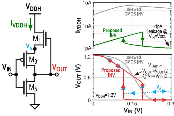
Fig. 2. Simulated dc transfer characteristics of the proposed DLS-based inverter operating from a 1.2-V supply with comparison to a skewed-sizing traditional CMOS inverter.
