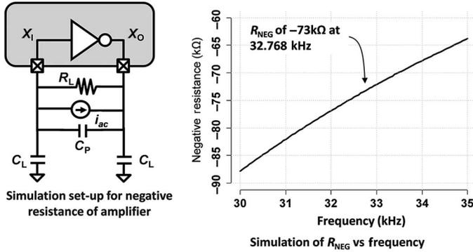
Fig. 2. Design method for the XTAL oscillator circuit.
