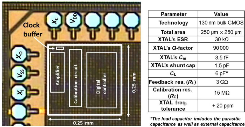
Fig. 20. Die photo of the XTAL circuit and parameters for the configuration in Fig. 1.
