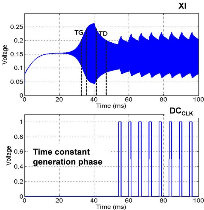
Fig. 12. Simulation of the duty-cycle XTAL oscillator at  $0.3 V_{DD}$ .
