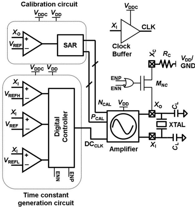
Fig. 11. Complete circuit architecture of the ULP XTAL oscillator.
