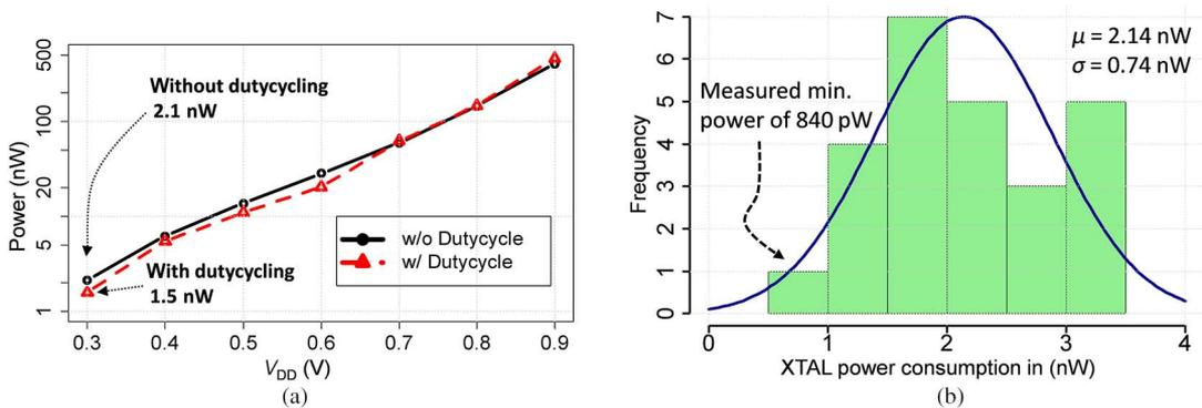
Fig. 16. Measured power consumption of XTAL.
