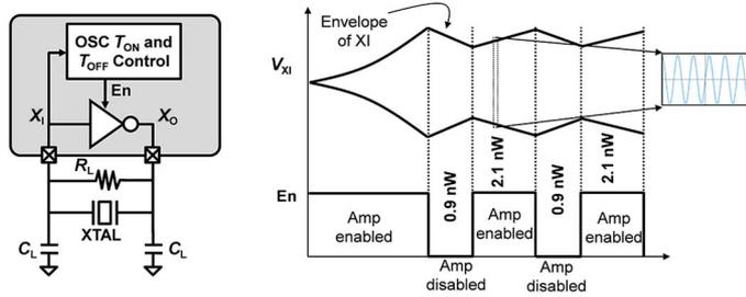
Fig. 7. Circuit diagram and operation of oscillator duty cycling.
