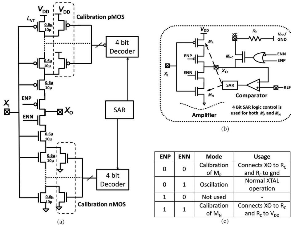
Fig. 4. XTAL oscillator amplifier design and calibration control.
