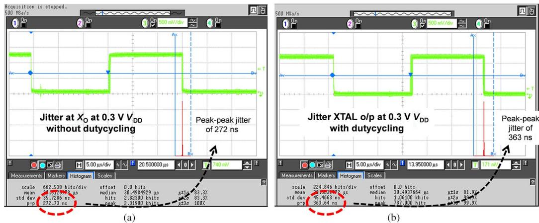
Fig. 15. Measurement of jitter at clock buffer out CLK without duty-cycling and with duty-cycling techniques.
