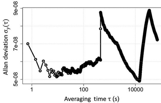
Fig. 18. Allan deviation measurement of the XTAL output with duty cycling at 0.3 V  $V_{DD}$  for approximately 20 h.
