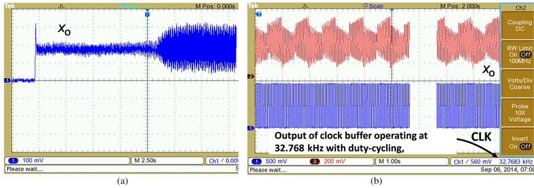
Fig. 14. Measured output waveform of the XTAL oscillator circuit. (a) Start-up of the XTAL oscillator at 0.4 V  $V_{DD}$ . (b) Measurement of the waveform at  $X_O$  with duty-cycling and producing the output clock at 32.768 kHz.
