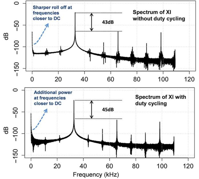
Fig. 13. Spectrum of XI with and without duty cycling.
