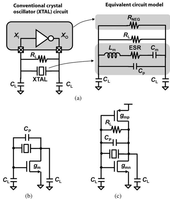
Fig. 1. (a) Conventional XTAL oscillator circuit and its equivalent representation. (b) Analysis of a three-point oscillator. (c) Practical implementation of XTAL oscillator with an inverter (push-pull oscillator).
