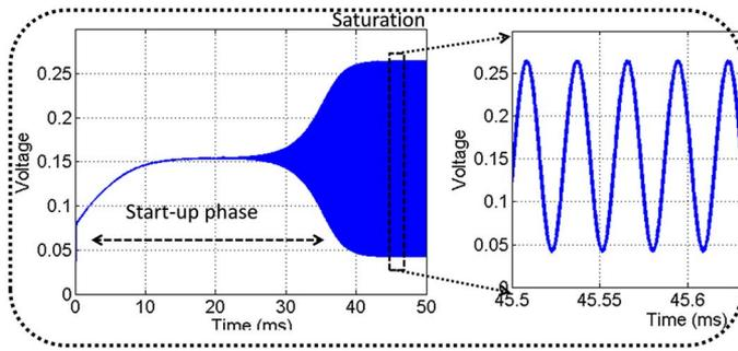
Fig. 6. Simulation result of the XTAL oscillator circuit operating at 0.3 V  $V_{DD}$  with a reduced  $Q$  XTAL resonator.
