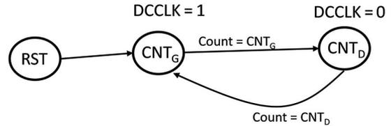
Fig. 10. Digital state machine for generating duty-cycling clock  $DC_{CLK}$ .
