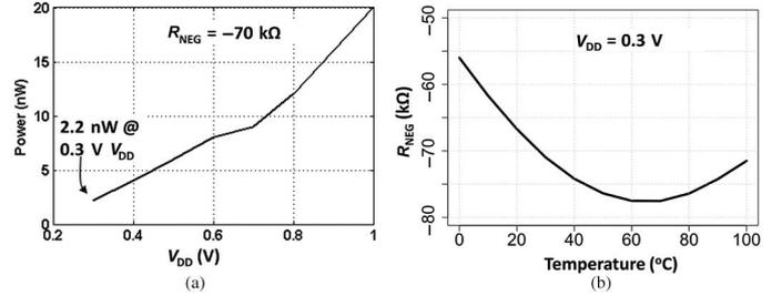
Fig. 3. (a) Simulation of XTAL oscillator power consumption across  $V_{DD}$  with a fixed negative resistance of amplifier at  $-70$  k $\Omega$ . (b) Simulation of negative resistance of the amplifier with temperature at 0.3 V  $V_{DD}$ .
