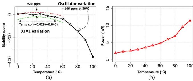
Fig. 17. Measured stability and power of the XTAL with temperature, w/o duty cycling, 0.3 V  $V_{DD}$  shows stability of 1.87 ppm/°C for a temperature variation of 0 °C–80 °C.
