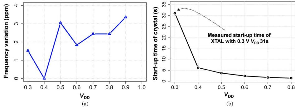
Fig. 19. (a) Measured frequency variation with  $V_{DD}$ . (b) Measured start-up time of XTAL with  $V_{DD}$ .
