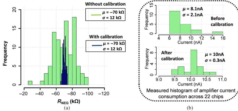
Fig. 5. Performance of the amplifier characteristics showing  $R_{NEG}$  across 100 point Monte Carlo simulation and its bias current measured across 22 chips before and after calibration.
