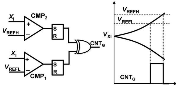
Fig. 8. Circuit to obtain the time constant for the growth of oscillation TG.
