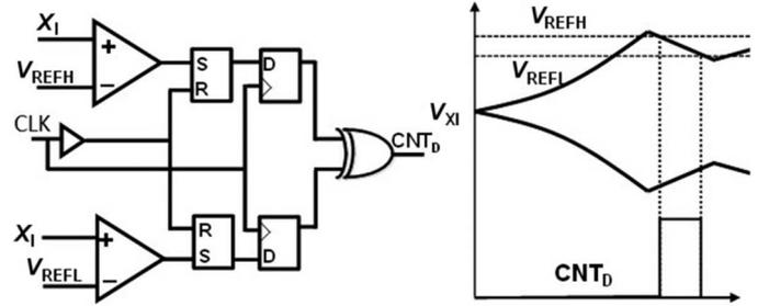
Fig. 9. Circuit to obtain the time constant for the decay of oscillation  $T_D$ .
