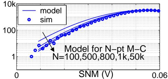
Figure 10: 50k-pt. M-C simulation for SNM with 4\*WL sized transistors. Model based on 1k-pt. M-C overlays model based on 50k-pt. M-C.
