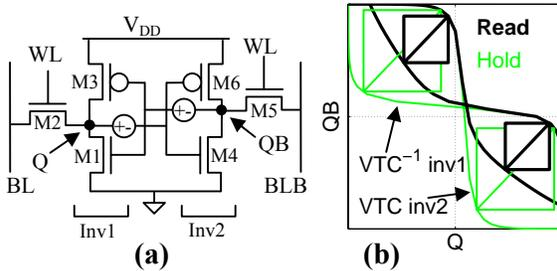
Figure 1: Schematic for 6T bitcell showing voltage noise sources for finding SNM (a). SNM plots (b).
