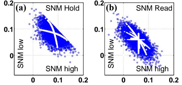
Figure 8: Scatter plots for SNM high vs. SNM low with single FET dependencies overlaid in white.
