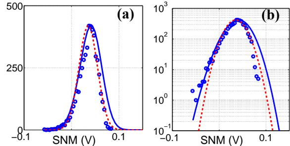
Figure 9: Histogram of SNM M-C simulation (circles) with normal PDF (dash) and PDF based on (6) (solid) over-laid. The semilog plot (b) shows that the PDF based on (6) matches the worst-case tail quite well.
