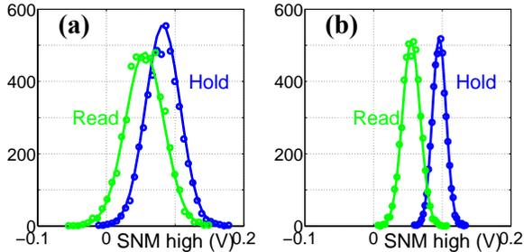
Figure 7: SNM high and low (not shown) for a min-sized cell (a) and for  $4*WL$  (b) is normally distributed with random  $V_T$  mismatch in all transistors.
