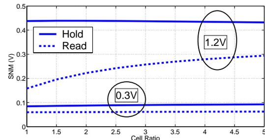
Figure 5: Cell ratio affects SNM less in sub-threshold
