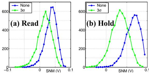
Figure 12: SNM M-C sims for mismatch on top of global variation (in legend).
