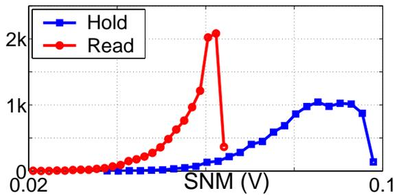
Figure 11: M-C simulation showing global variation impact on SNM for minimum sized bitcell.
