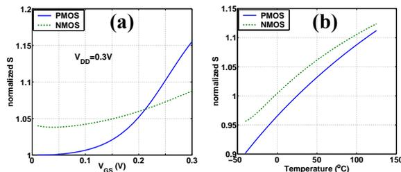
Figure 3: Changes in sub-threshold slope ( $S$ ) versus  $V_{GS}$  (a) and temperature (b).
