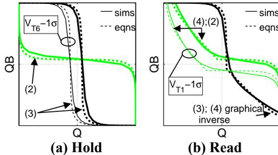
Figure 2: 1<sup>st</sup>-order VTC equations versus simulations.
