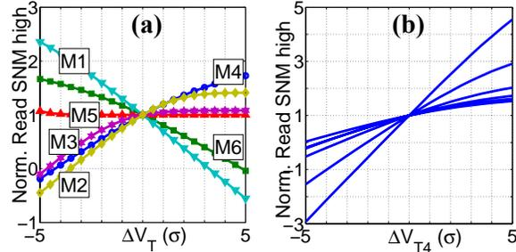
Figure 6: Dependence of SNM high on single FETs is nearly linear (a) but slope depends on other  $V_T$ s (b).
