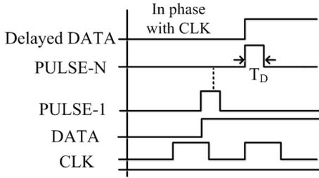
Fig. 5. Timing Diagram and Phase Detection
