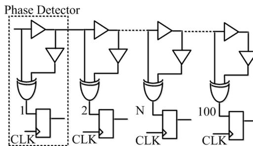
Fig. 4. Delay Line with Phase Detectors
