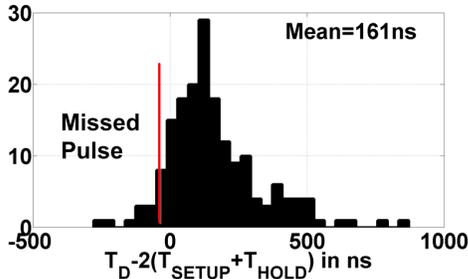
Fig. 6. Design Margin for Pulse Generator
