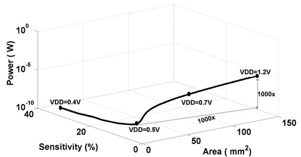
Fig. 9. Power Area and Sensitivity tradeoff
