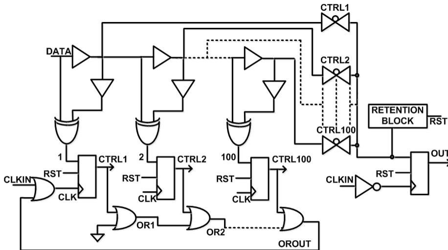
Fig. 12. Complete Circuit Diagram of CDR
