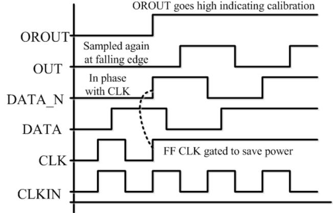
Fig. 11. Timing Diagram
