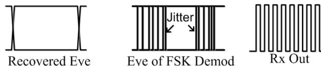
Fig. 3. Received Signal at Various Stages
