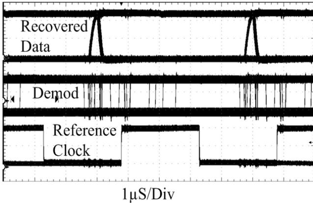
Fig. 13. Measured Data recovery from FSK Demod with 2μs Jitter
