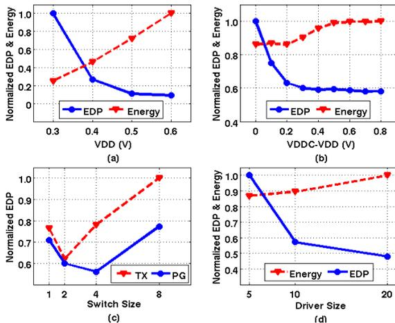
Fig. 7. Measured path with length 40 for (a)  $V_{DD}$  optimization (b)  $V_{DDC}$  optimization @  $V_{DD} = 0.4V$  (c) switch size optimization @  $V_{DD} = 0.4V$  (d) driver size optimization @  $V_{DD} = 0.4V$
