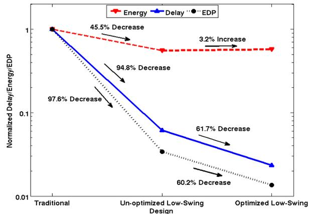
Fig. 6. Comparison of the normalized delay, energy, and EDP @  $V_{DD} = 0.4V$
