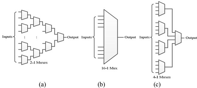
Fig. 4. Schematic of different CB topologies: (a) full multiplexer (b) 1-stage multiplexer (c) 2-stage multiplexer
