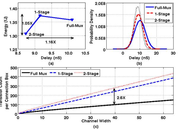
Fig. 5. Comparison of different CB topologies (a) ED curve @  $V_{DD} = 0.4V$  (b) variation @  $V_{DD} = 0.4V$  (c) area
