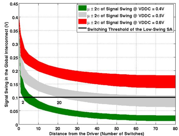
Fig. 3. Range of signal swing for varying path length from Monte Carlo (MC) simulations with PG interconnect compared to the  $V_M$  of SA @  $V_{DD} = 0.4V$
