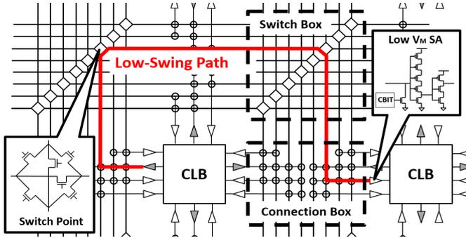
Fig. 1. Basic structure of low-swing interconnect
