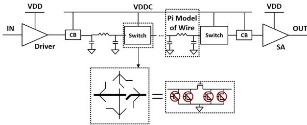
Fig. 2. Diagram of the global interconnect path model
