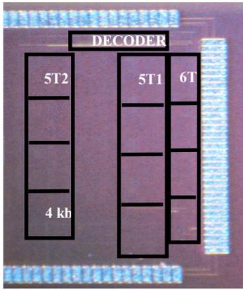
Fig. 8: Die photo of section of the fabricated 45 nm chip containing 32kb of 5T and 16kb of 6T SRAM.
