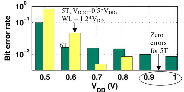
Fig. 11: Writability of 5T vs. 6T at lower  $V_{DD}$  for a 4 kb bank. Both 5T and 6T are stable for read to below 0.5 V for these banks.
