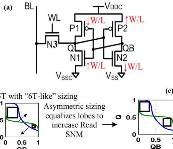
Fig. 1: (a) 5T bitcell schematic. (b) Read Static Noise Margin (RSNM) for 5T with 6T-based sizing. (c) RSNM for 5T with asymmetric sizing
