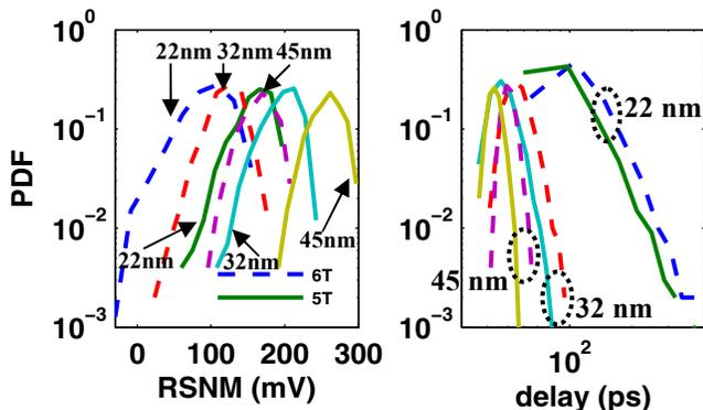
Fig. 3: Effect of scaling (using predictive models [10]) on (a) RSNM and (b) read delay.
