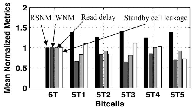
Fig. 4: Asymmetric sizing used as a knob to trade off cell area with RSNM, WNM (with write assist for 5T), read delay, and leakage. All bitcells have the same area. For 5T standby leakage, the average of the leakage for the cell storing ‘0’ and ‘1’ is shown.
