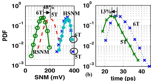
Fig. 2: 45nm (a) SNM & (b) Read Delay for 5T vs. 6T, from a 1000 point Monte Carlo Simulation at TT, 27 °C, 1 V.
