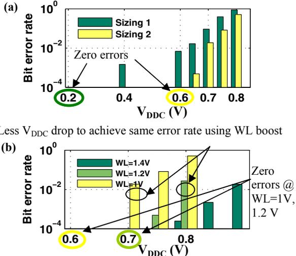
Fig. 10: Measured impact of (a) cell sizing and, (b) WL boosting on the effectiveness of the  $V_{DDC}$  reduction write-assist, on a 4 kb bank.
