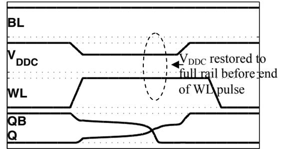
Fig. 6: Timing for  $V_{DDC}$  collapse write-assist.
