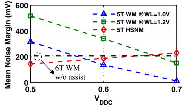
Fig. 7: Retention margin of half-selected cells limits  $V_{DDC}$  collapse. Boosting WL fixes this problem by allowing for a smaller drop in  $V_{DDC}$  for the same WNM.
