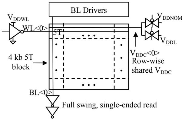
Fig. 9: Schematic of Write Assist implementations on chip
