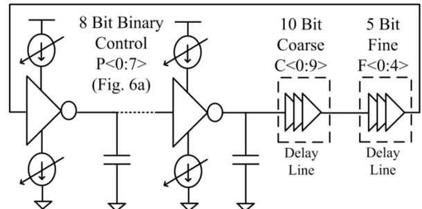
Fig. 7.  $\text{Osc}_{\text{CMP}}$  DCO Architecture
