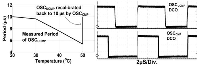
a) Recalibration of  $OSC_{UCMP}$  with  $OSC_{CMP}$  b) Measured Waveform of DCO outputs at 100kHz after re-calibration
