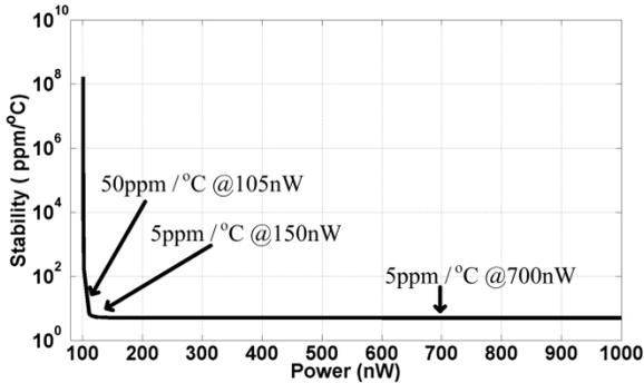
Fig. 14. Measured Power/Stability tradeoff for 1°C/Sec. temperature change
