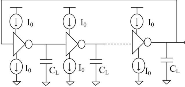
Fig. 3. Current controlled Ring Oscillator
