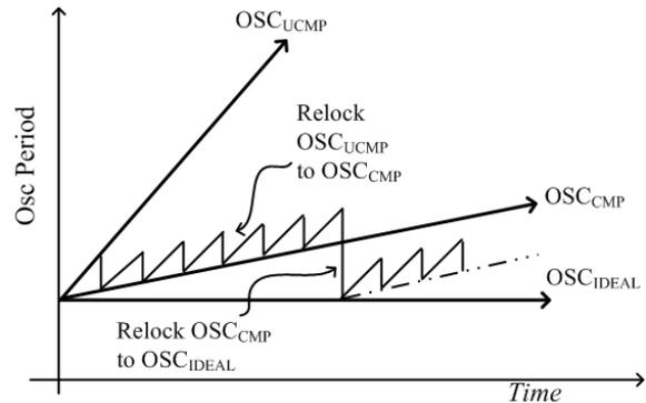
Fig. 1. Scheme of re-locking low stability oscillator to achieve high effective stability
