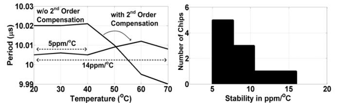
a) Measured Clock period of OSC<sub>CMP</sub>
