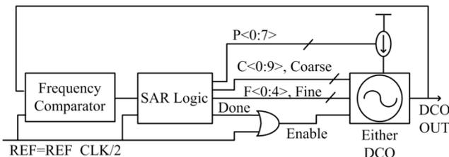
Fig. 10. Fast Locking circuit for DCO using binary search
