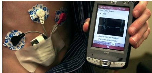
Figure 3 – ECG sensor sending waveform over a Bluetooth connection to a PDA base station.
