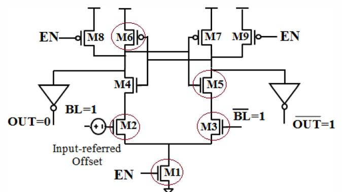
Figure 2. Sense amp condition after it latches according to the input-referred offset, when M2 has higher  $V_T$  than M3.
