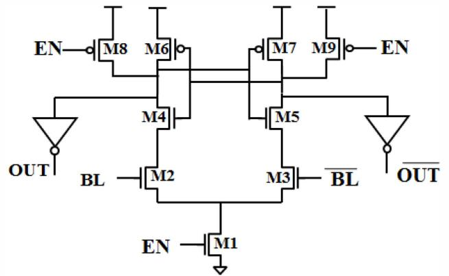
Figure 1. Latch-based sense amp
