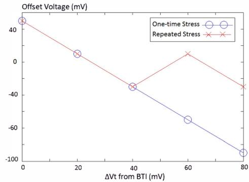
Figure 4. Effect of One-time and repeated BTI stress on the offset voltage
