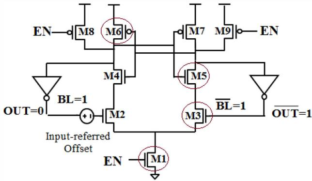
Figure 3. Feeding the output back to the input during stress to avoid stressing the weaker input device.
