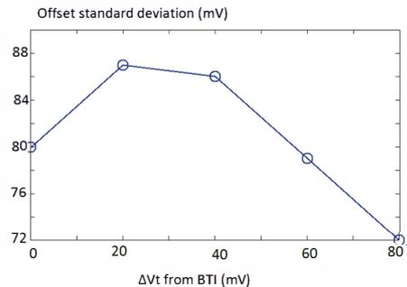
Figure 6. Standard deviation of the offset voltage after each stress step
