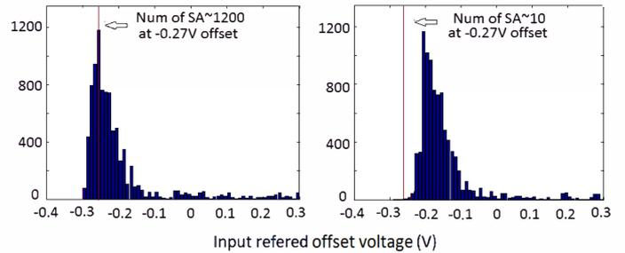
Figure 9. a. Initial distribution of the measured offset voltage
