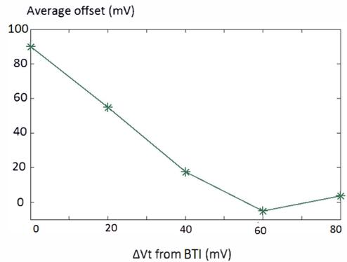
Figure 5. Average value of the offset voltage after each stress step
