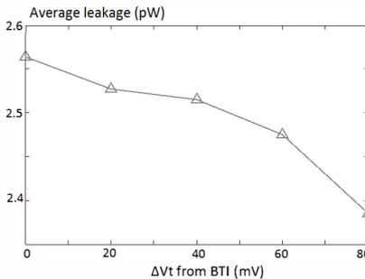
Figure 8 Average leakage after each stress step
