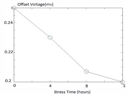
Figure 10. Average measured offset voltage after each stress time.
