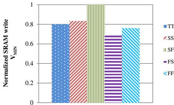
**Figure 16: Normalized SRAM write  $V_{MIN}$  for 100 million SRAM bits with 99% yield constraints at 85C.**
