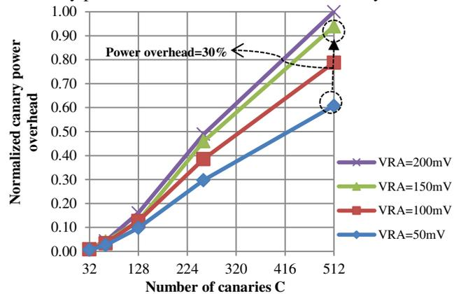
Figure 13: Normalized canary total power overhead vs. number of canaries  $C$  with  $N=512Kb$  SRAM for different  $V_{RA}$  voltages at 1GHz  $TT_{85C}$  corner.
