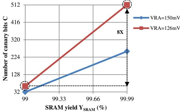
**Figure 6:** Trend of C vs.  $Y_{SRAM}$  with 100 million SRAM bitcell at constant  $P_{fc}=10^{-5}$  for different  $V_{RA}$  voltages @ TT\_85C.
