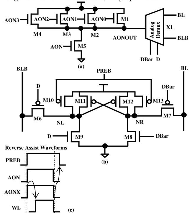
**Figure 8:** (a) Canary SRAM reverse assist circuit. (b) Canary write driver. (c) Reverse assist waveforms.
