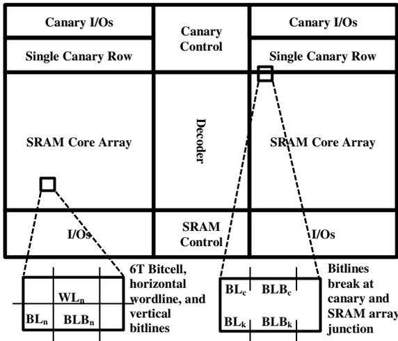
Figure 9: Block diagram of the canary SRAM inside SRAM macro (not in scale).
