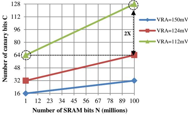
**Figure 5:** Trend for C vs. N with 95% SRAM yield at constant  $P_{fc}=10^{-5}$  for different  $V_{RA}$  voltages @ TT\_85C.
