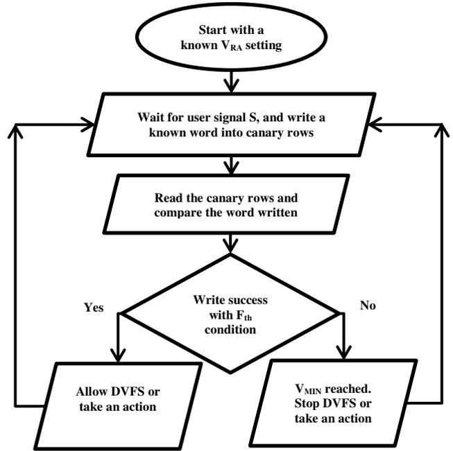
Figure 10: SRAM  $V_{MIN}$  tracking algorithm using canary SRAMs with reverse assist.
