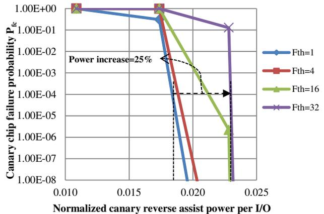
Figure 14: Canary chip failure probability vs. normalized reverse assist total power for increasing  $F_{th}$  conditions at 1GHz  $TT_{85C}$  corner ( $C=128$ ).
