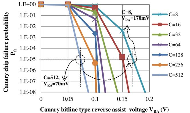
**Figure 4: Canary chip failure probability vs. reverse assist voltage for 1 million SRAM bitcells with 95% yield @ TT\_85C.**
