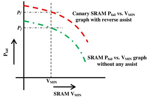
**Figure 3: Methodology to calculate canary chip failure probability.**
