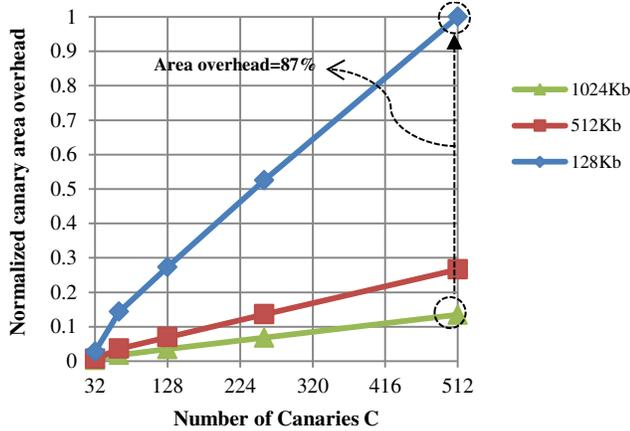
Figure 11: Normalized canary area overhead vs. number of canaries for different SRAM sizes.
