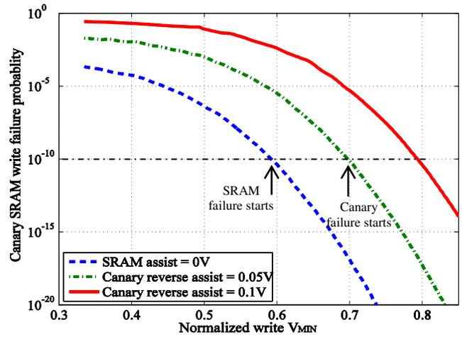
Figure 2: Canary SRAM dynamic write failure probability vs. normalized write  $V_{\text{MIN}}$ .
