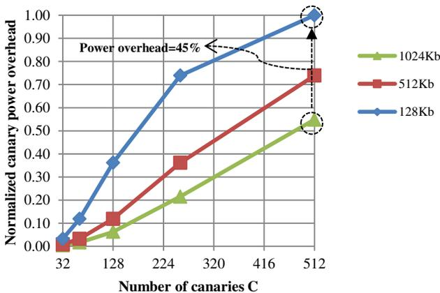
Figure 12: Normalized canary total power overhead vs. number of canaries  $C$  with constant  $V_{RA}=50mV$  for different SRAM sizes at 1GHz  $TT_{85C}$  corner.
