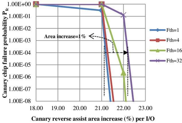
**Figure 15: Canary chip failure probability vs. canary reverse assist area increase per I/O for increasing  $F_{th}$  conditions ( $C=128$ ).**
