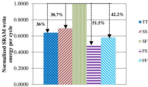
**Figure 17: Normalized SRAM write energy per cycle at  $V_{MIN}$  for 100 million SRAM bits with 99% yield constraints at 85C.**
